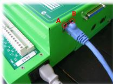
LAN Cable Connection
