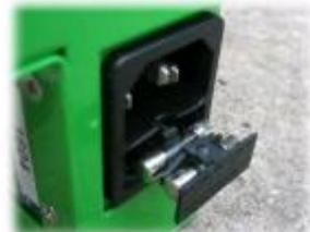
IEC power socket showing fuse access
