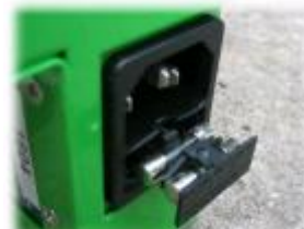
IEC power socket showing fuse access
