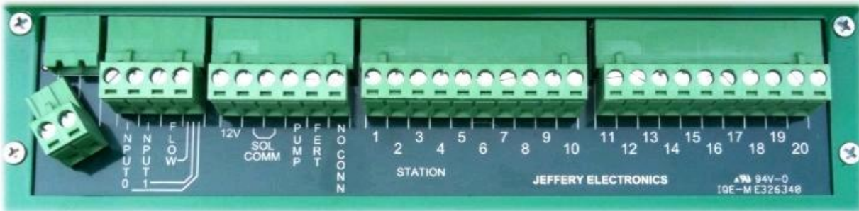
Cloudmaster terminal blocks showing first block unplugged
