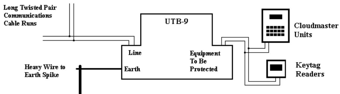
Mains supply spike protection can also be useful although not usually as crucial as protection on long comms cables. A power point with built-in protection is better than nothing, but an externally wired device, such as the DSF-6A-275V, has much higher surge current capability. This device also requires a heavy ground cable to a good ground spike.
